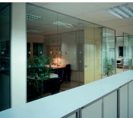
This super-slim full-height single glazed partitioning system uses a high-quality aluminium framework only 25mm wide, which accepts glass of 10mm up to 12.8mm thick using standard tear-off glazing gaskets. Thicker glass can be used if required. As with all other Finesse and Crystal systems, the sections are clip-together, and are designed to substantially reduce on-site installation time, particularly where transitions to either double
